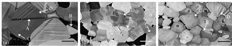
Fig. 4. Backscattered electron micrographs of the barium titanate samples studied, showing twinning in the grains: (a) BaTiO 3 , (b) (Ba,Ca)TiO 3 , (c) (Ba,Ca,Sr,Pb)TiO 3 . Arrows indicate twin types: A, double annealing twins; B, single annealing twins; C, parallel (ferroelectric) twins and D, tapered (deformation) twins (scale bars = 5 \mu\text{m} ).
